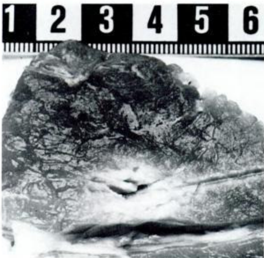
Fig. XVII: 4. Piece of meat (moossteak) after local diathermic production of heat over an electrode perfused with saline solution. The cut surface through the boiled tissue is approximately 2.5 \times 1.5 cm and grey-white. Diathermia over a dry electrode produces a small, black region of dry tissue, which easily breaks conductivity of the circuit.
